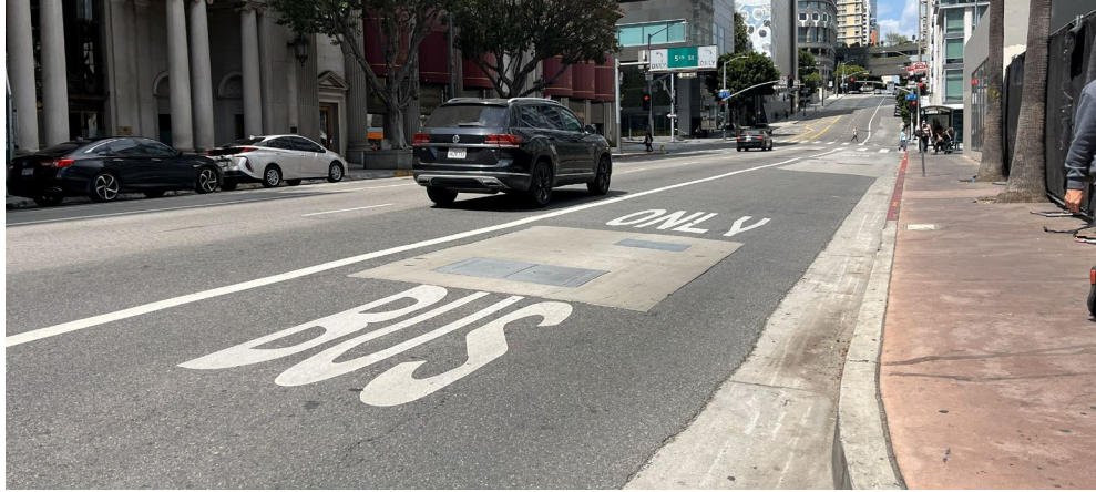
Photo 25 Reconfigure a street to add a “bus only” lane prioritizing/promoting mass transit flow
